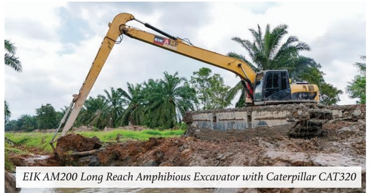
out directly on soft ground with minimal disturbance, reducing the need for temporary access materials while maintaining stable and controlled operations. The long-reach capability further supports efficient shaping and rehabilitation of the waterway, limiting repeated machine movements along the channel.
