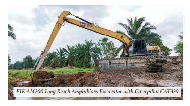
out directly on soft ground with minimal disturbance, reducing the need for temporary access materials while maintaining stable and controlled operations. The longreach capability further supports efficient shaping and rehabilitation of the waterway, limiting repeated machine movements along the channel.
