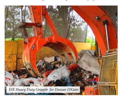
When it comes to recycling and material sorting, speed, precision, and durability are essential. The EIK Heavy-Duty Grapple, seen here paired with a Doosan DX200, is built to thrive in high-cycle environments—whether you're handling scrap, construction debris, or general waste. This fixed-type hydraulic
