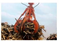
Orange Peel Grab (also known as Cactus Grab) comes in 2 variants, hydraulic and mechanical, and both are designed for heavy duty operations, suitable for handling scrap metal, rock, wood chips, garbage, etc. A rotator can be added as an optional feature, assuring efficient and precise positioning of the load in the pile or over a truck. It can handle virtually any scrap, waste or recycling job with confidence.
