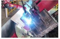
Mass production model of buckets are welded by the latest robotic welding machine. We supply a full range of buckets to suit excavators up to 200 metric tons (440,000 lbs) operating weight. Buckets are designed differently, either in the type of material used or the profile of the bucket to suit different applications for the best possible productivity, fuel economy and durability.
