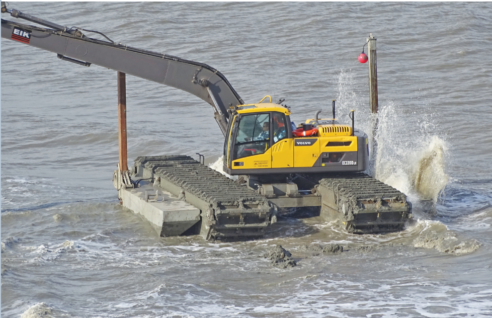
Supplementary pontoons can be added on each side to enhance stability.
