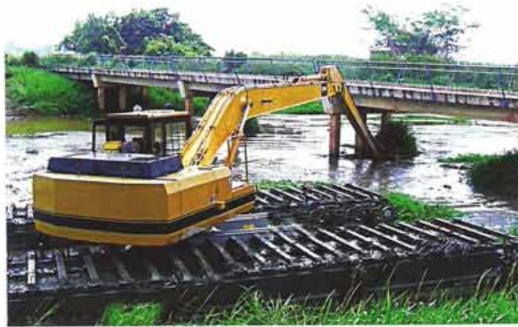
Completely self-propelled, the Amphimaster can access all terrains and yet requires minimum supporting transportation or hoisting equipment.
