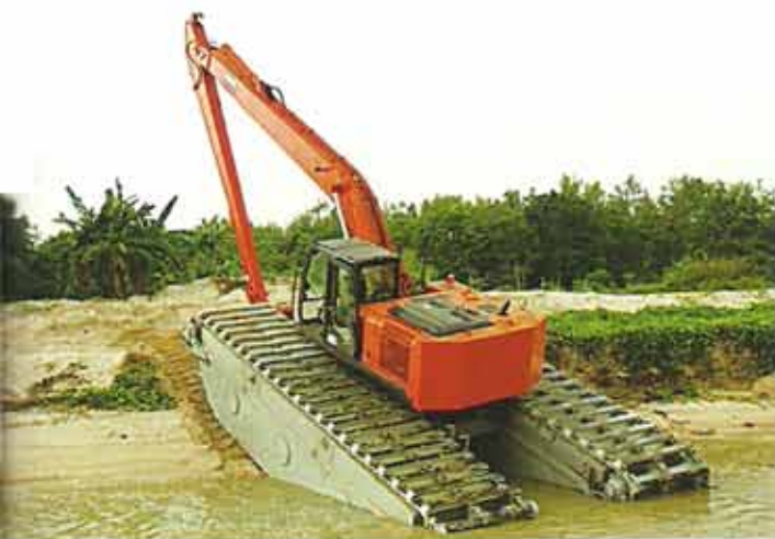
Completely self-propelled, the Amphimaster can access all terrains and yet requires minimum supporting transportation or hoisting equipment.
