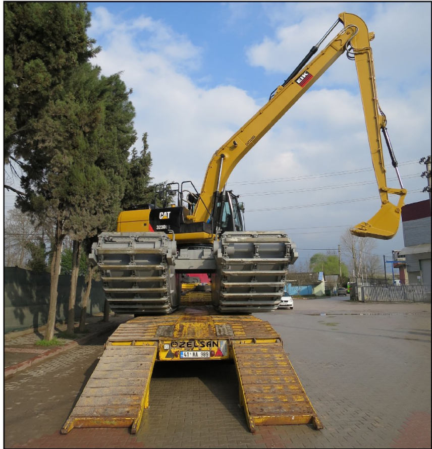
This EIK model AM200-3E undercarriage holding a CAT 323D2 excavator in the retracted position of 15 feet nine inches is a stable load on a trailer eight feet six inches wide. The distance between the pontoons is four feet one inch. The extended width is 20 feet seven inches, which would require a special trailer and special permits to transport by road. Photo location is in Turkey.
