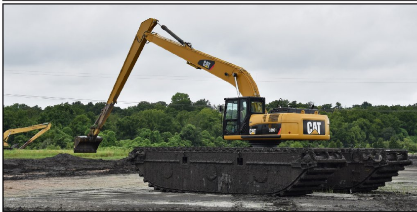
A CAT329D on an EIK AM300 undercarriage working an ash pond dewatering in Kansas City, Missouri.
