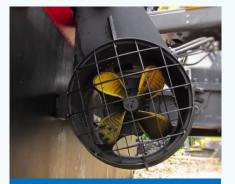
Propeller on Pontoon Undercarriage
