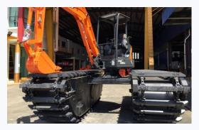
Model AM60, another leading product designed to cater for the 4-5 ton class excavator segment. This machine size is very much in demand for cleaning small canals and waterways. The entire machine can be easily haul around in cities, as well as tight and narrow rural access path.
