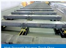
High Strength Polymer Track Shoe Getting Ready for Field Test
