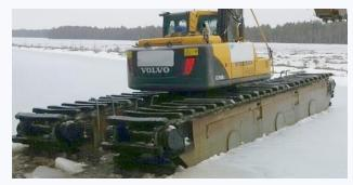
The picture on the right is the condition of the polymer track shoes working in the field for more than 5000 hours. No replacement is required.
