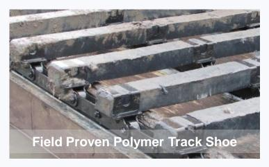
We have been relentlessly pursuing better materials to improve our product quality. The polymer material use for the track shoes is one of the significant improvement made through selection of material, and our confidence is backed by extensive field test data.
