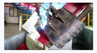
For standard buckets produce in high volume, we invested in robotic welding system to ensure consistency, quality and productivity.
