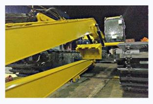
All done in-house, the EIK team worked around the clock to put the AM200 Amphibious Excavator together, attached with upper body CAT320D. To meet the deadline, our team put in great effort to assemble everything and was able to deliver the final product on time.
