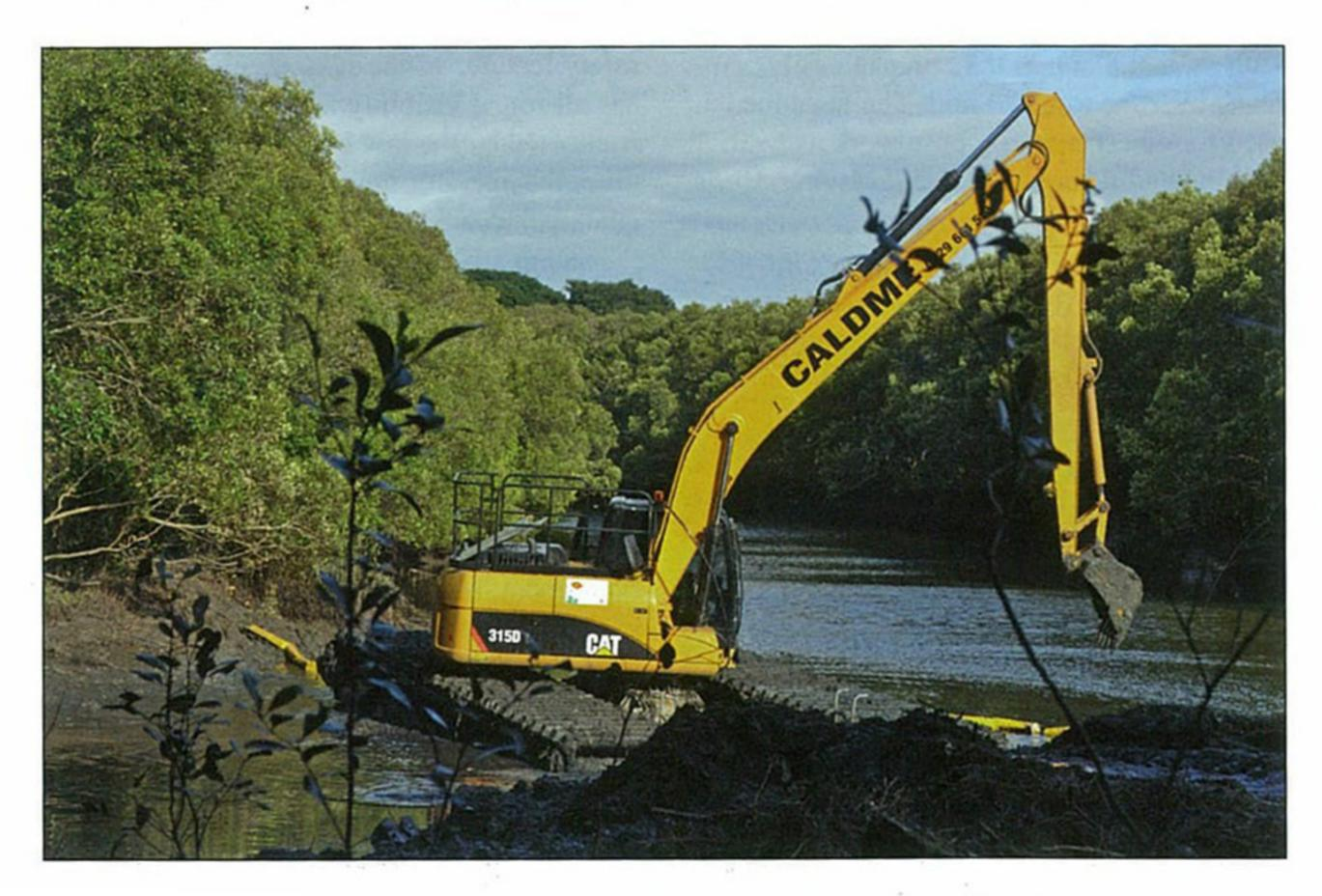
ALDME is Tamborine-based contractor specialising in long reach excavators, and the "Great Dane" excavator – all tracks and boom – is a machine you'll see nowhere else in Australia: a Cat 315D excavator with an amphibious undercarriage and long reach boom [there are other amphibious excavators but not of this size].
